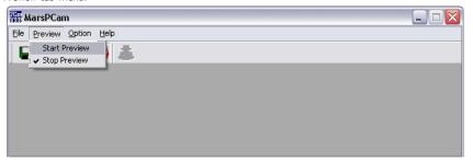
**Step 9:** Press the button to capture the image from the camera. Otherwise click on "Capture Frame" from the Option tab menu.
